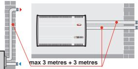
The splitter makes it possible to solve all problems related to the position of the fume flue. Intake and exhaust ducts are separate and can cover distances up to 3 m each.  $90^{\circ}$  elbows make it possible to move the ducts sideways, as the total length of 3 m must be reduced by 50 cm for each elbow used.
