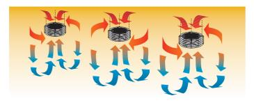
If several units are to be installed, the directions of rotation should be alternated in order to blend air more efficiently.
